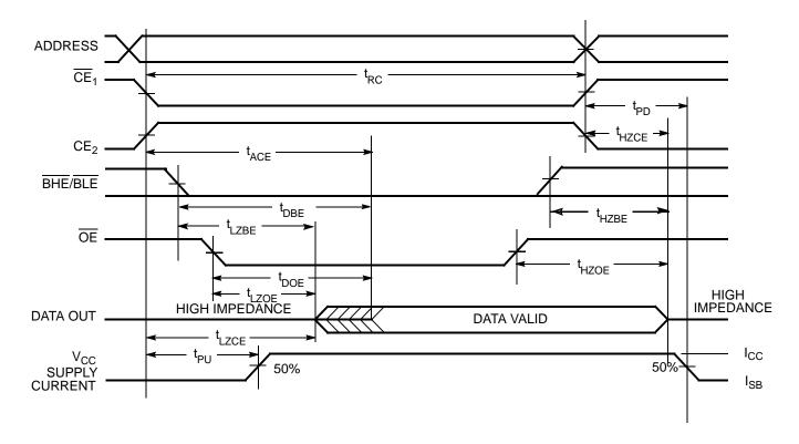
19. The device is continuously selected.  $\overline{OE}$ ,  $\overline{CE}_1 = V_{|L}$ ,  $\overline{BHE}$  and/or  $\overline{BLE} = V_{|L}$ , and  $\overline{CE}_2 = V_{|H}$ . 20.  $\overline{WE}$  is HIGH for read cycle.
